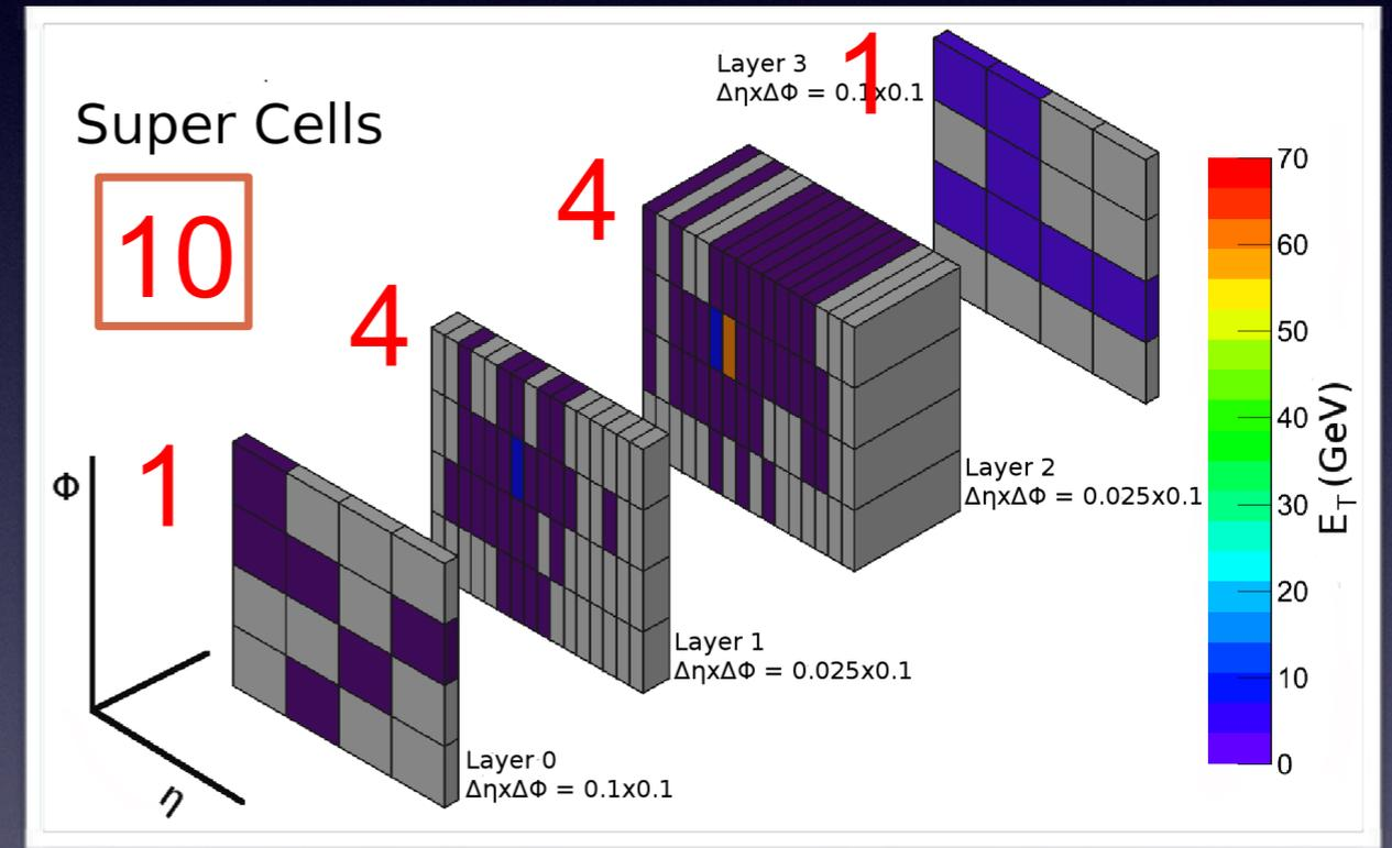
Trigger towers  $\rightarrow \Delta\eta\Delta\Phi=0.1 \times 0.1$
