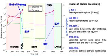
Hysteresis loss The hysteresis loss is compared with that obtained using the ITER formula [8] for fully penetrated strands:
