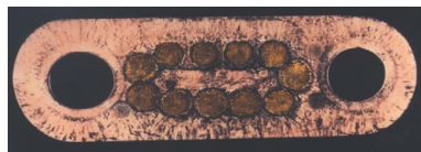
RW Nb 3 Sn conductor of T15 TF coil
