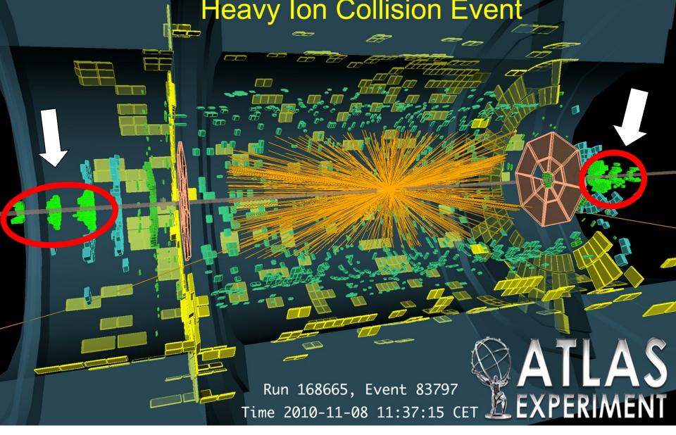
2 Forward Calorometers (FCal) are used for RP approximation: 3.2< $|\eta|$ <4.9. Tracks from Inner Detector are used for flow harmonics determination:  $|\eta|$ <2.5
