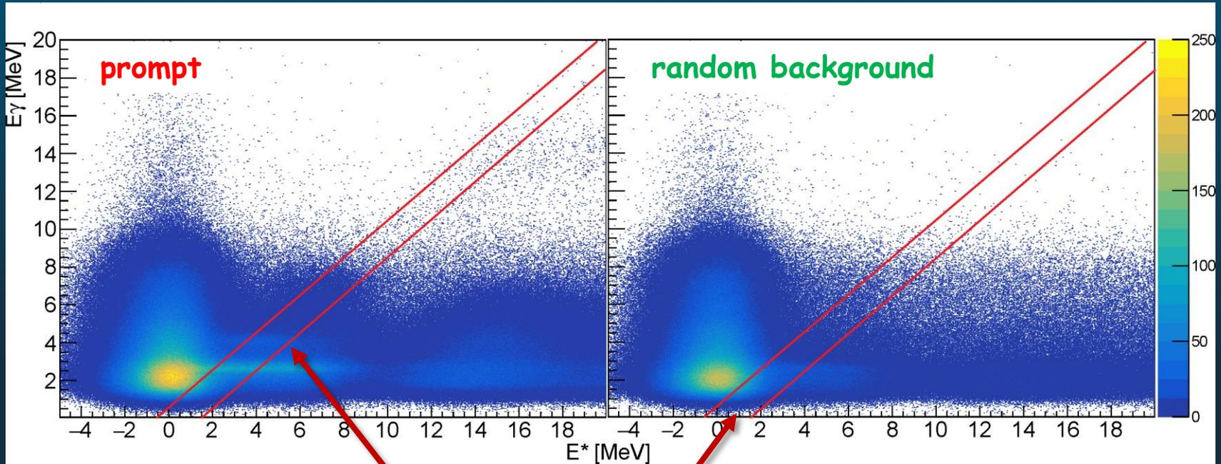
decay to the ground state ( $[E_\gamma + 0.5 - E^*] \leq 1 \text{ MeV}$ )
