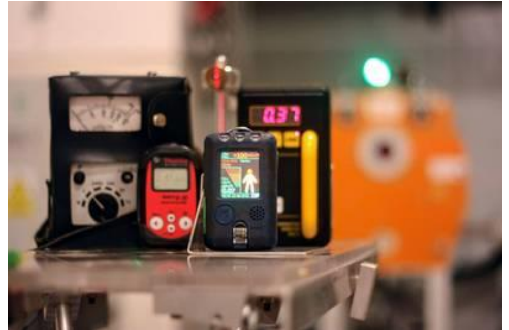
Calibration of radiometers at Cs-137 calibration bench
