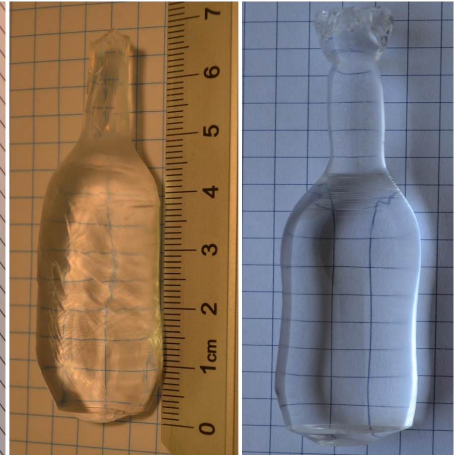
Our LiF crystals obtained by Czochralski method
