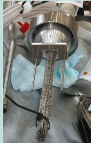
Electrical connection of 81 triplets
