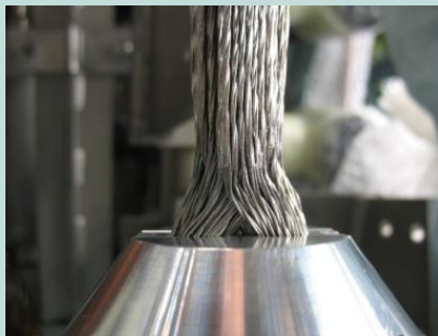
Electrical connection of 81 triplets
