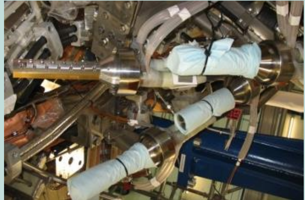
Connected triplets squizzed with clamps and covered by stainless steel caps
