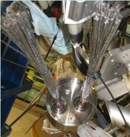
Electrical connection of 81 triplets
