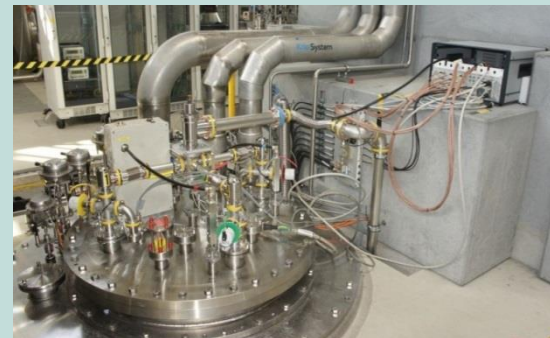
Cavity test-stand, cryostat (left) and electronic racks (right)
