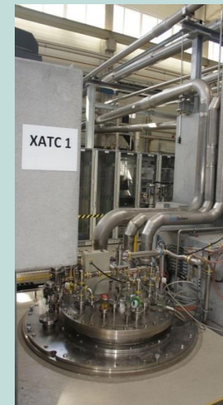
Cryogenics operator's control panel for test cryostat (left) and subcooler box (right) at AMTF. Cavity cryostat at AMTF
