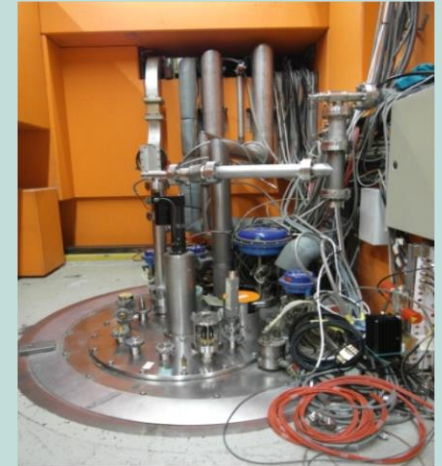
Insertion of the cavity into the vertical cryostat
