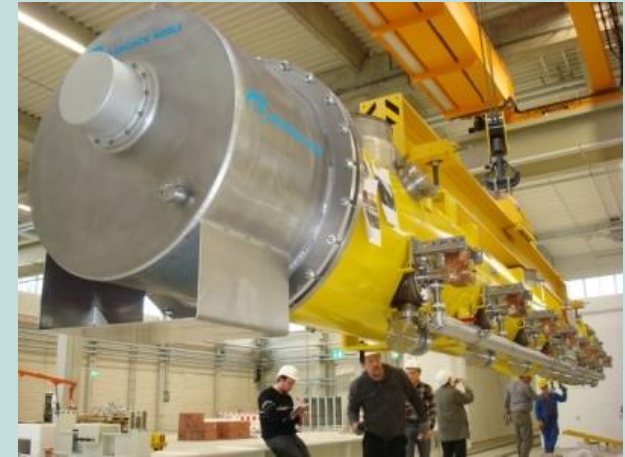
XFEL cryomodules tests
