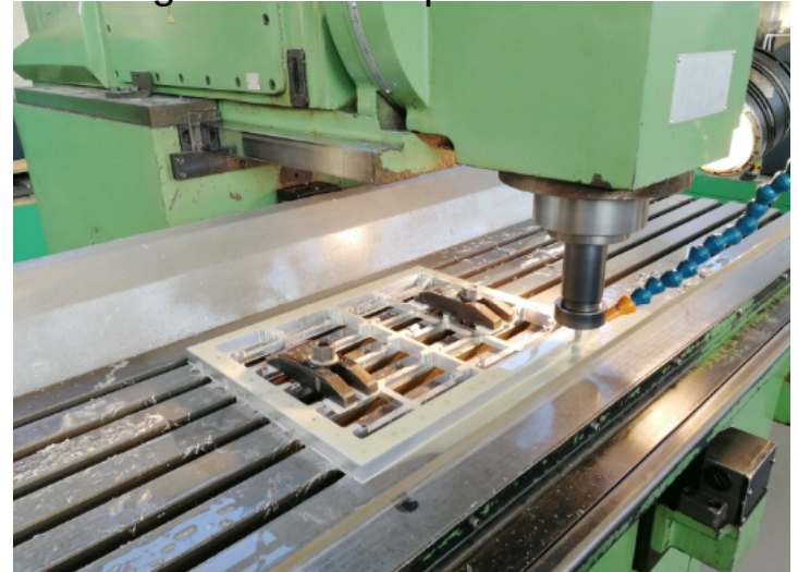
MicroMegas stiffeners production in IFJ DAI
