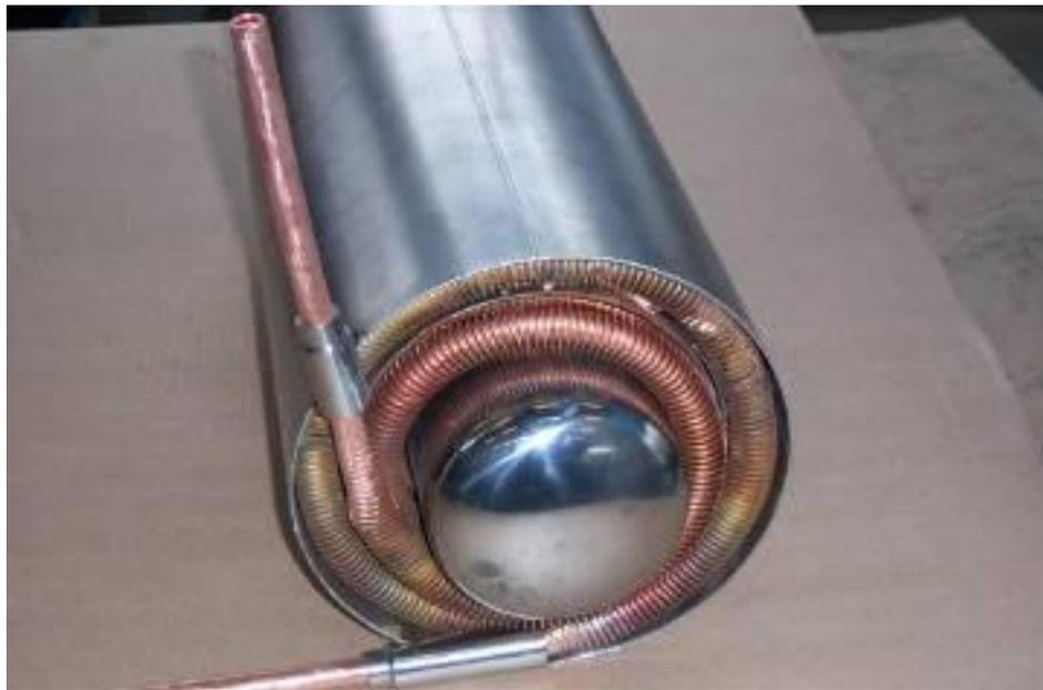
LPHE double coil after installation
