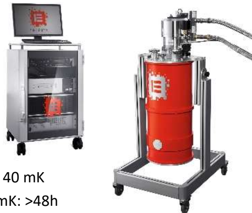
X-Ray Spectrometer (working temp. 65 mK)
