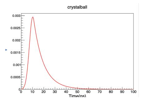
Further, time spread due to PMT transit time (per photo-electron) from the following distribution
