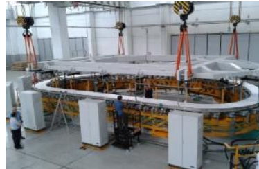
6. DOUBLE PANCAKE GROUND INSULATION
