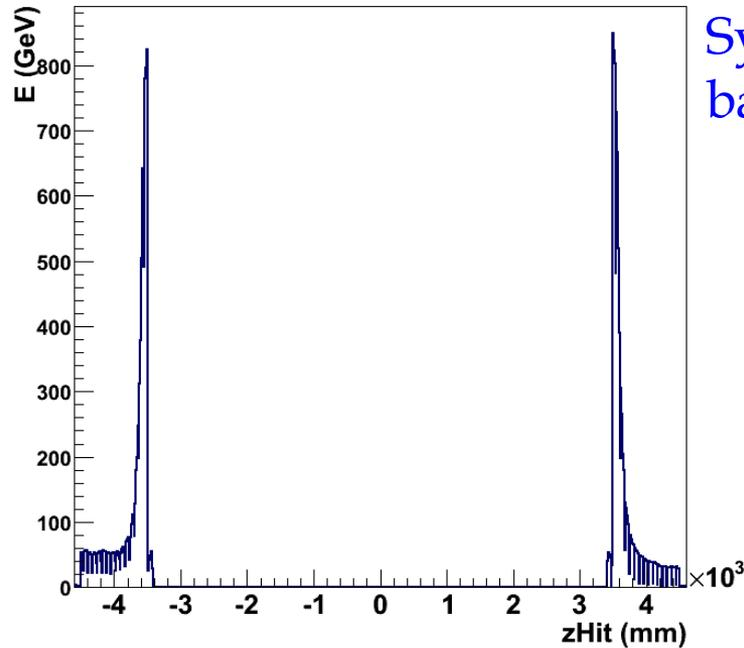
Symmetric energy deposition in the backward and the forward QD0
