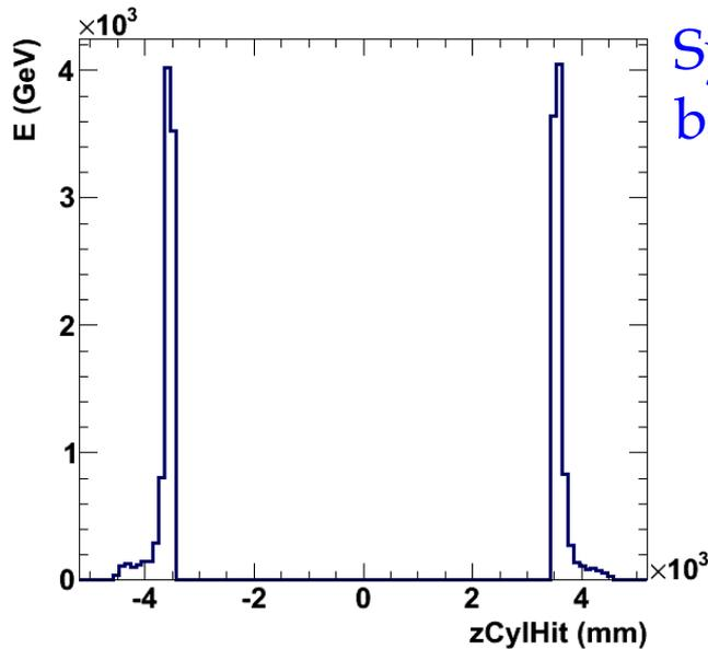
Symmetric energy deposition in the backward and the forward cylinders
