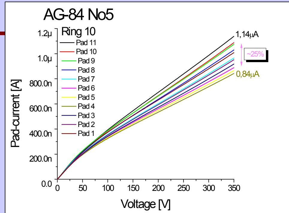
Rad. Hard Silicon sensor tests at the NLCTA beam (150-200 MeV electrons)
