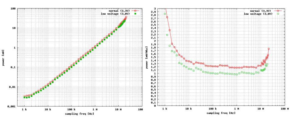
Presently power consumption about 1-1.5 mW/MHz at worst case (Nyquist input frequency, output buffers)
