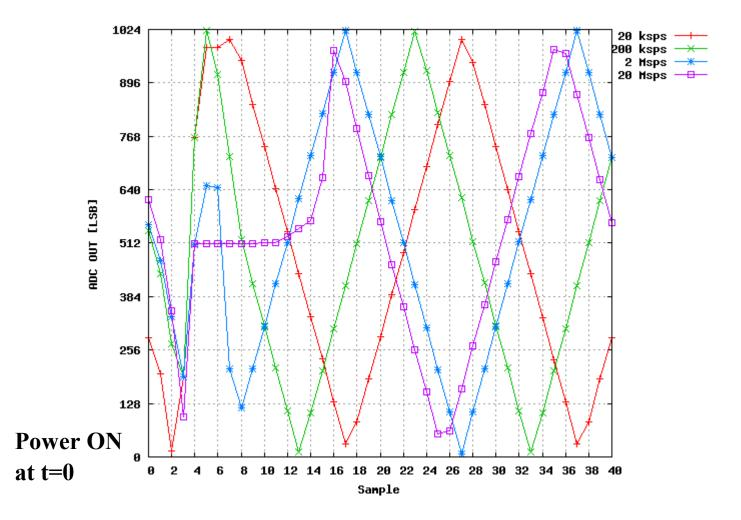
Depending on sampling frequency 8-16 clocks needed for switching\_ON
