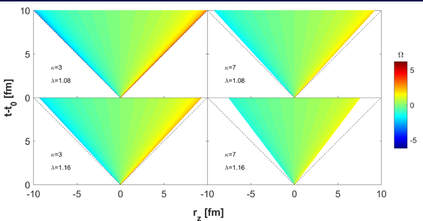
**Figure 3.** Fluid rapidity  $\Omega$  maps in the forward light cone from our new, longitudinally finite solutions are shown for  $\kappa = \varepsilon/p = 3$  (left column) and for  $\kappa = 7$  (right column) evaluated for the acceleration parameters  $\lambda = 1.01, 1.02, 1.04$  and  $1.08$  (from top to bottom rows) corresponding to nearly flat and with increasing  $\lambda$ , gradually narrowing rapidity distributions.
