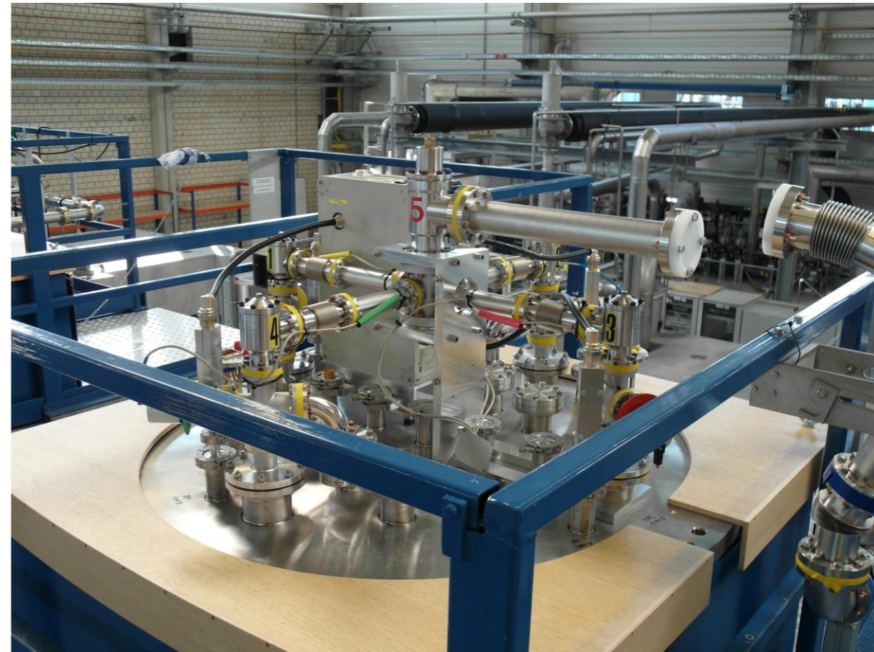
Insertion of the cavity into the vertical cryostat
