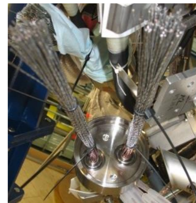
Electrical connection of 81 triplets
