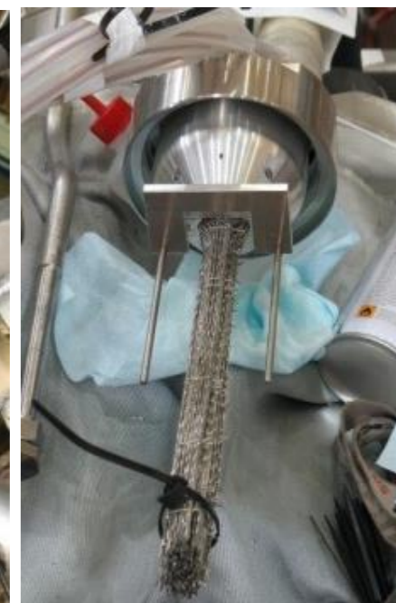
Electrical connection of 81 triplets
