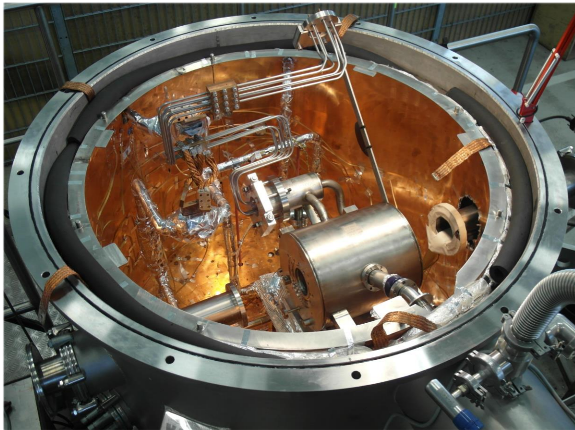
XFEL quadrupole inside the cryostat vessel
