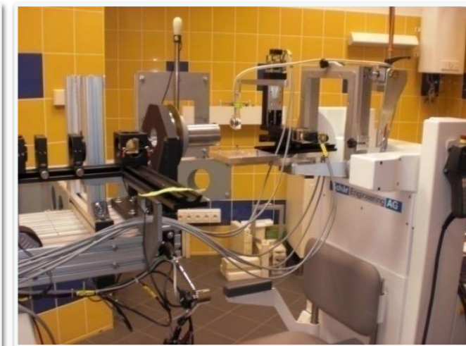
Fixtures of XYZ scanner and water phantom on the ETC (Eye Therapy Chair)
