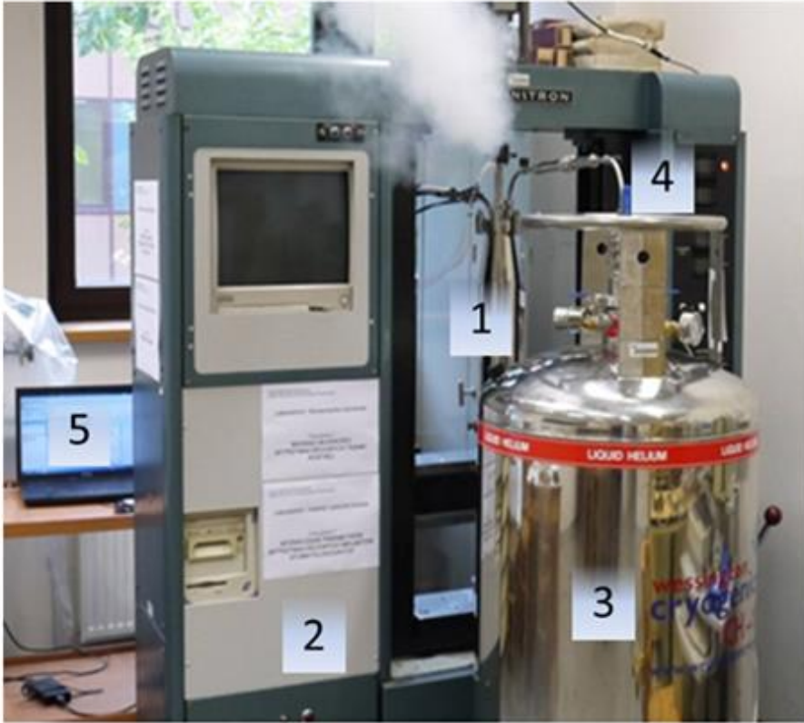
Experimental set-up for: a) uniaxial tensile tests; b) combined loading; c) cryostat with equipment (1- cryostat, 2- tensile test machine, 3- cryogen dewar, 4- cryogen transfer line, 5- DAQ system, 6- clip-on extensometers, 7- specimen, 8- force transducer, 9- thermistor)
