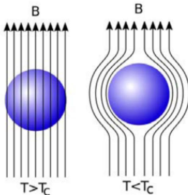
Fig. 2 . A superconductive ball, cooled down in an external magnetic field. For  $T < T_c$  the magnetic field  $B$  is expelled from the sample.
