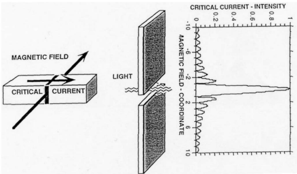
Analogy of a Josephson junction in a magnetic field and light diffracted in a single slit.
