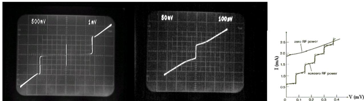
**Figure:** Current-voltage characteristics of tunneling and weak-link Josephson junction (without and in microwave field).
