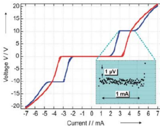
Current-voltage characteristic of a 10-V series array consisting of 69,632 SNS Josephson junctions under 70-GHz microwave irradiation. The width of the constant-voltage step is above 1 mA, which guarantees correct AC operations.
