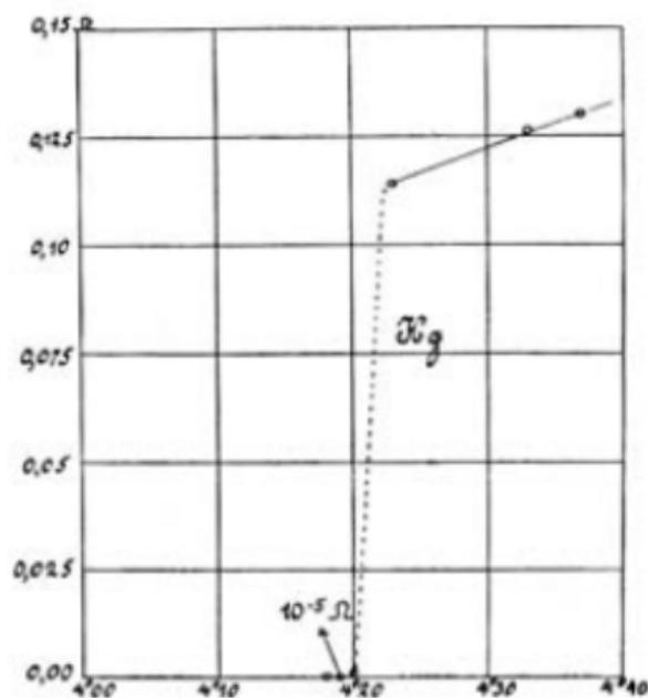
Fig. 1. Kamerlingh Onnes' measurement of the resistance of a mercury sample denotes the detection of superconductivity in the year 1911.
