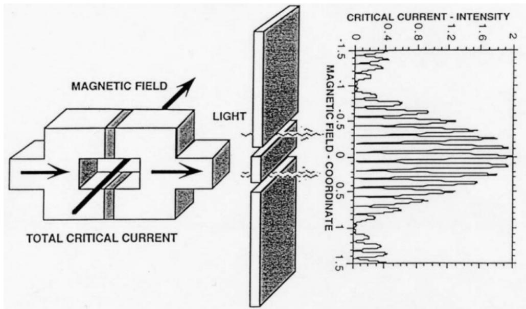
Analogy of a SQUID in a magnetic field and light interfering through two slits.
