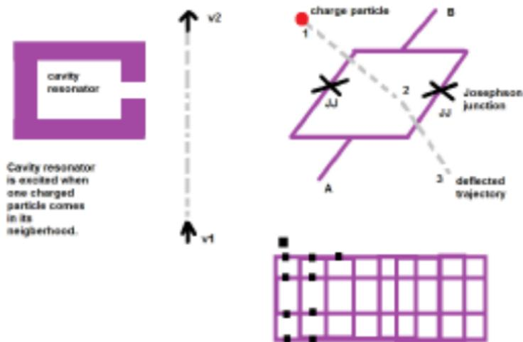
Principle of excitation of resonant cavity by charged particle.
