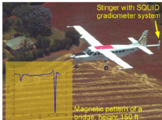
... Air borne SQUID system for geophysical sounding (IPHT Jena).
