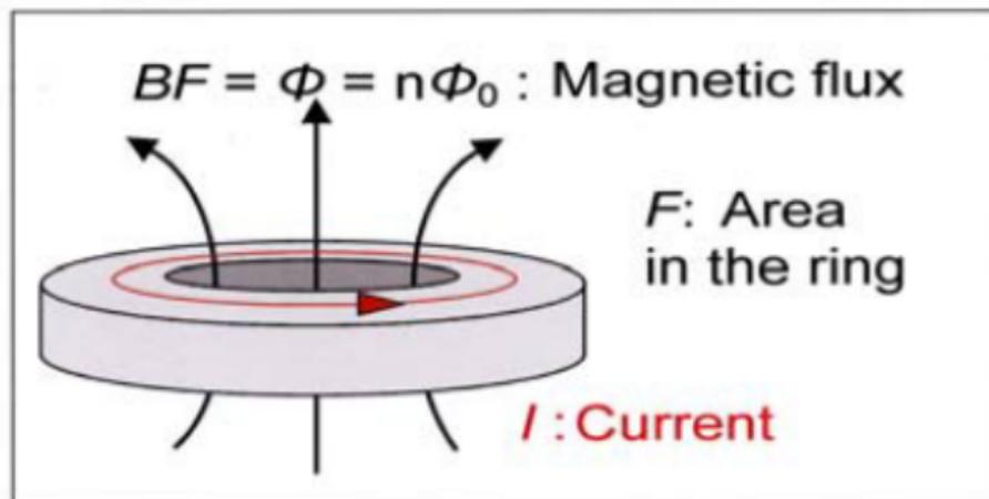
Fig. 3. In a current carrying superconductive ring the magnetic flux as product the magnetic field and the ring area is quantized in integer multiples of  $\Phi_0 = h/2e$ .
