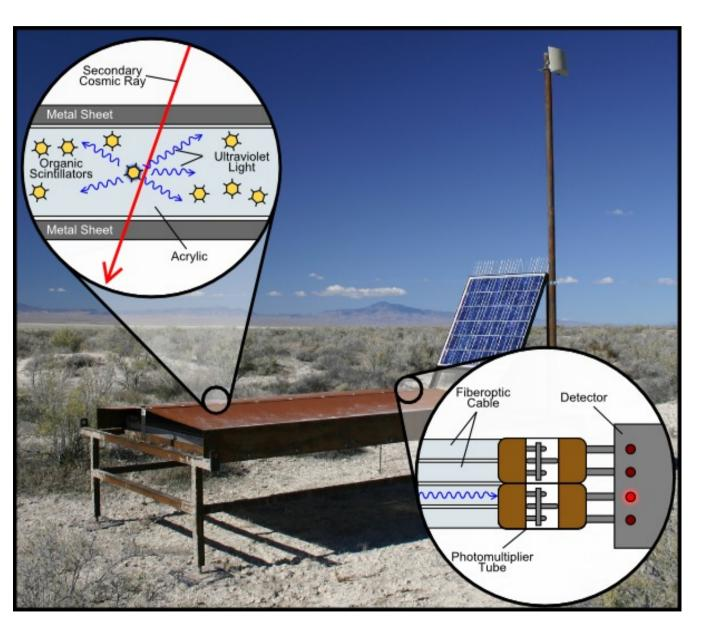
Easier to handle than water no fluid components higher light yield  $\rightarrow$  smaller volume
