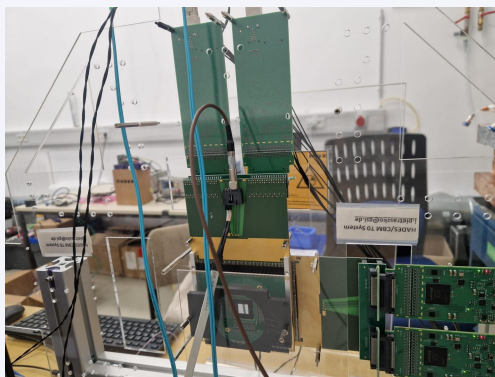
START diamond detector (GSI)
