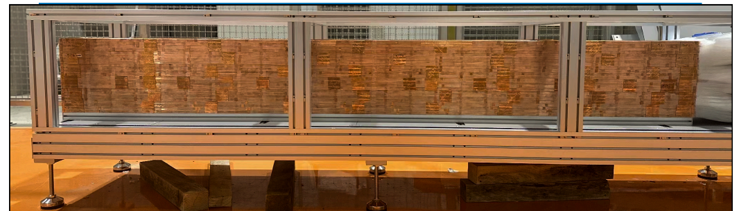
Figure 29: Barrel region of the dual-readout calorimeter, with a few towers tall for visualization purposes (left). Backside of one tower with the assembly of tubes and the support structure around them, forming one tower (right).
