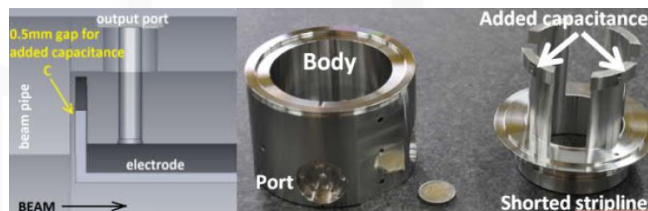
(Beam position monitor)
