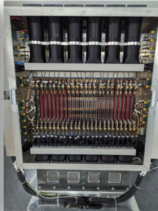
Detector complete, installed, and initial testing with cosmoics done
