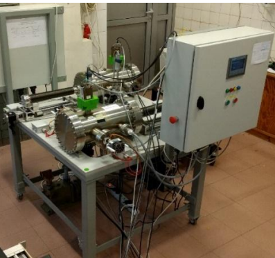
Dedicated test stand for feedthrough and diamond detectors thermal stress tests at IFJ PAN
