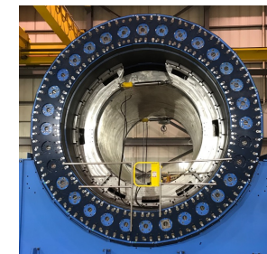
Barrel HCal Fe/Sc sandwich, \sim 3.5\lambda (sPHENIX re-use)
