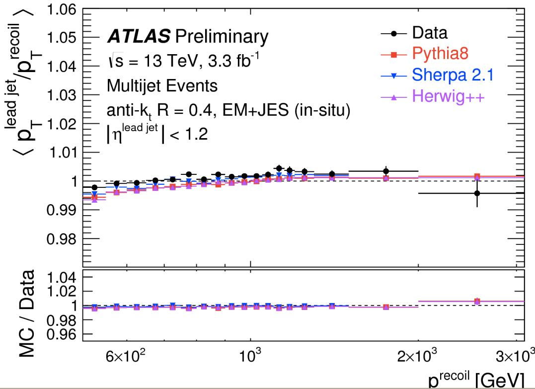
Multijet balance distributions for data and MC simulation using anti- $k_t$  R=0.4 jets, calibrated with the EM+JES and 2012 *in situ* corrections applied
