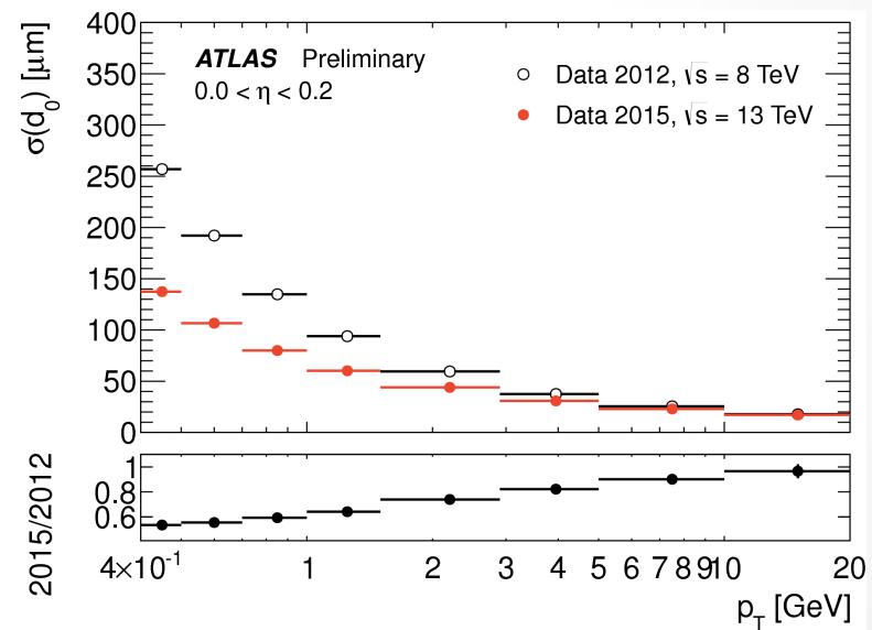
Unfolded trans. impact parameter resolution in 2015 w/ IBL compared to that in 2012 w/o IBL
