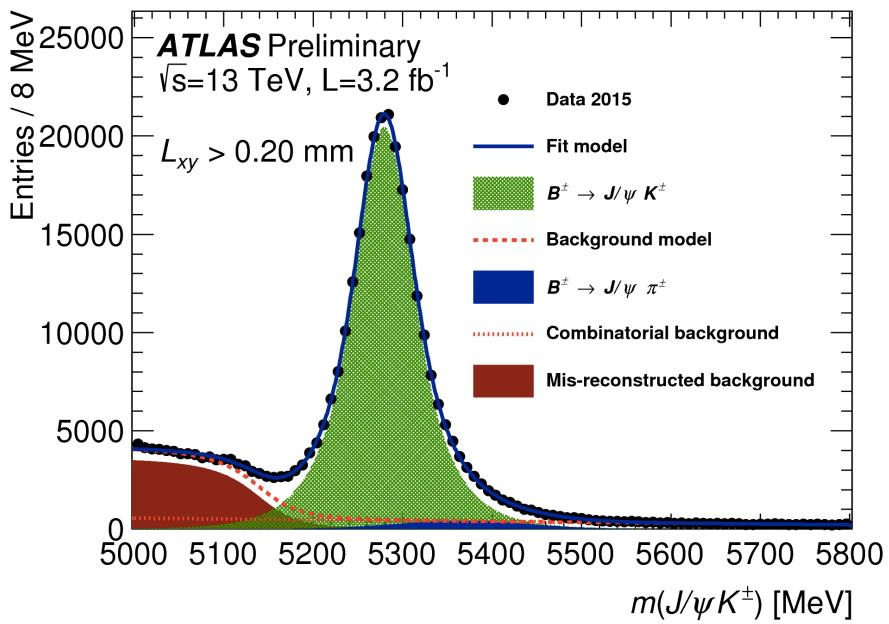
Alignment and tracking performance check with reconstructed  $B^\pm$  mass
