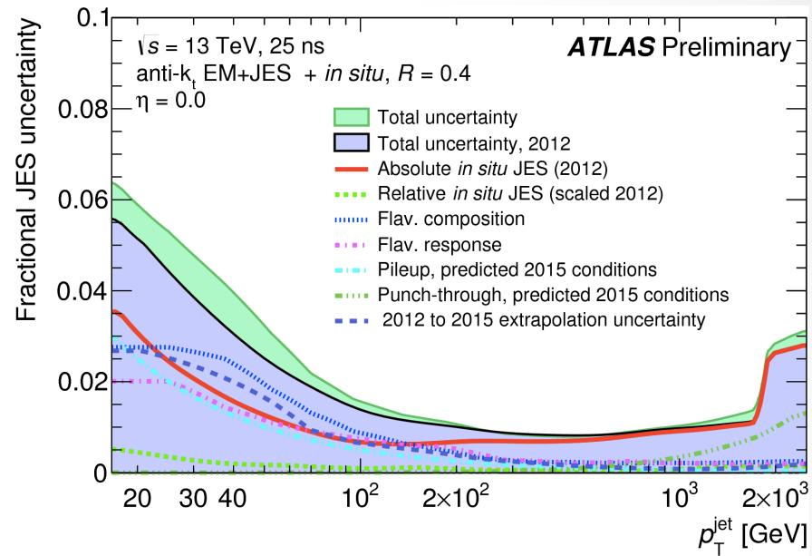
**Jet energy resolution** uncertainties estimated for 2015 data with 25 ns bunch spacing as a function of jet  $p_T$  for jets of  $\eta = 0$
