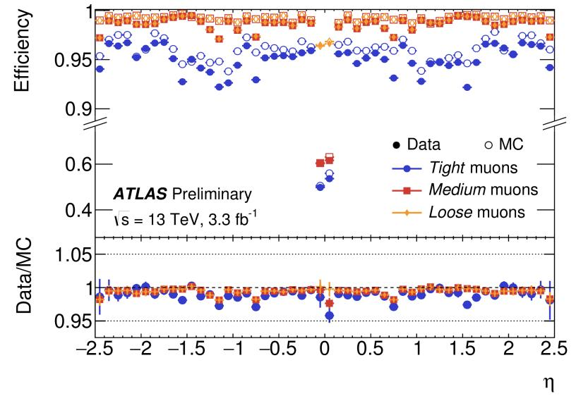
Muon reconstruction efficiencies for the Loose/Medium/Tight identification algorithms measured in  $Z \rightarrow \mu^+\mu^-$  events as a function of  $\eta$  for muons with  $pT > 10 \text{ GeV}$ .
