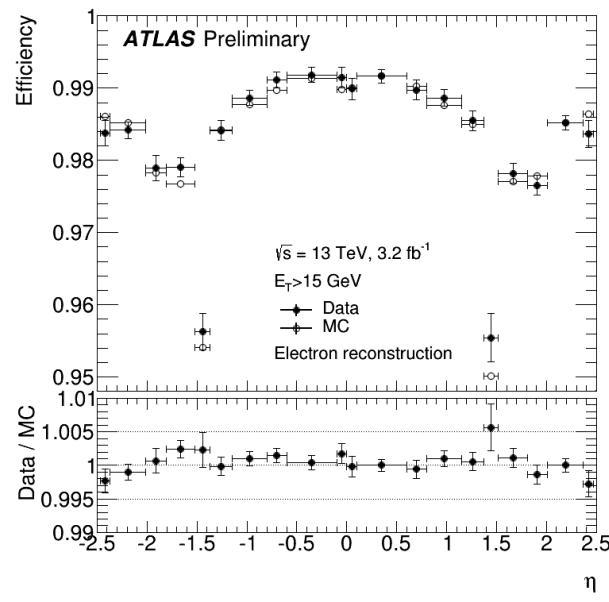
Electron reconstruction efficiencies are measured by  $Z \rightarrow ee$  candidates
