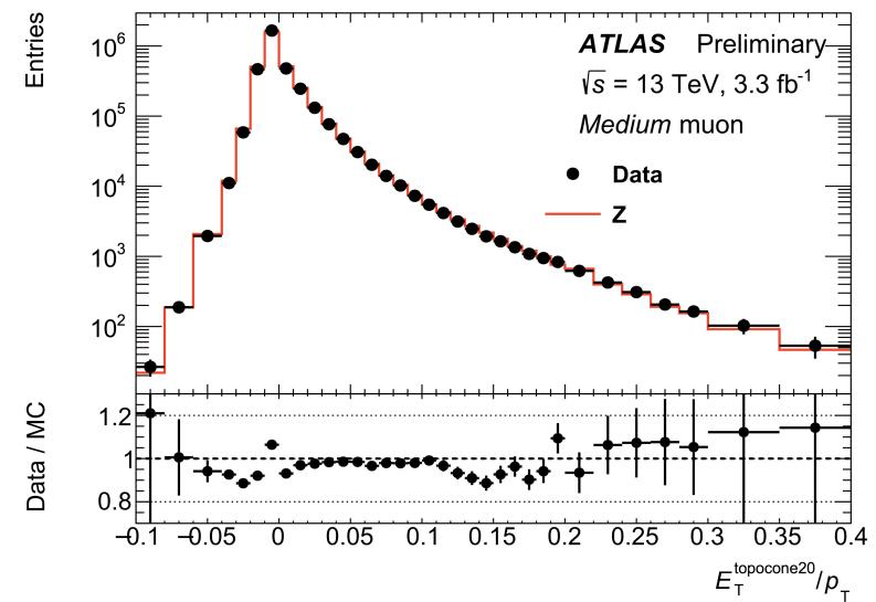
Distributions of the track-based (left) and the calorimeter-based (right) isolation variables, divided by the muon  $p_T$  measured in  $Z \rightarrow \mu^+\mu^-$  events.
