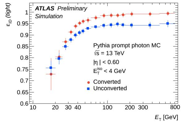
Expected Photon efficiency in Run 2 based on MC.
