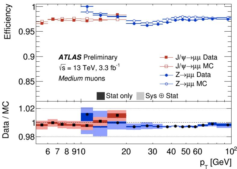
Muon reconstruction efficiencies for the Medium identification algorithm measured in  $J/\psi \rightarrow \mu^+\mu^-$  and  $Z \rightarrow \mu^+\mu^-$  events as a function of the muon momentum.
