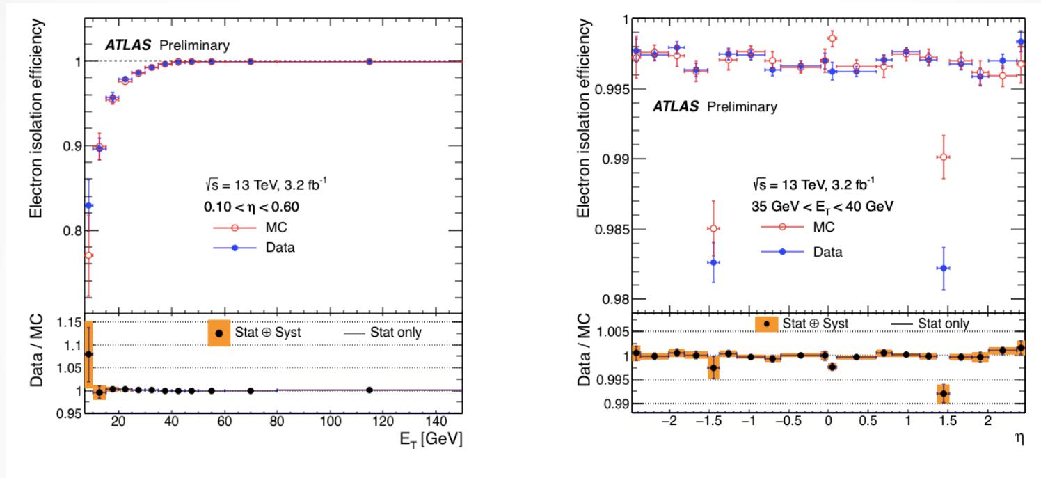
Efficiency of the isolation requirement for tight electrons
