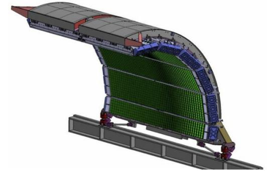
• EMCAL Pb-scintillator sampling calorimeter:
