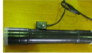
Cherenkov radiator in a light guide
