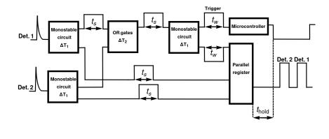
$t_s$  - signal length.  $t_w$  - window length.  $t_{hold}$  - time after which data is read.  $\Delta T_{1,2}$  - delays. Jerzy Pryze Tests of small shower array 8/32
