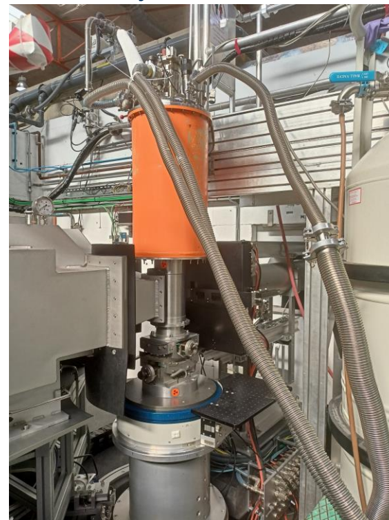
Fig. 7 Sample environment with “Orange cryo”
