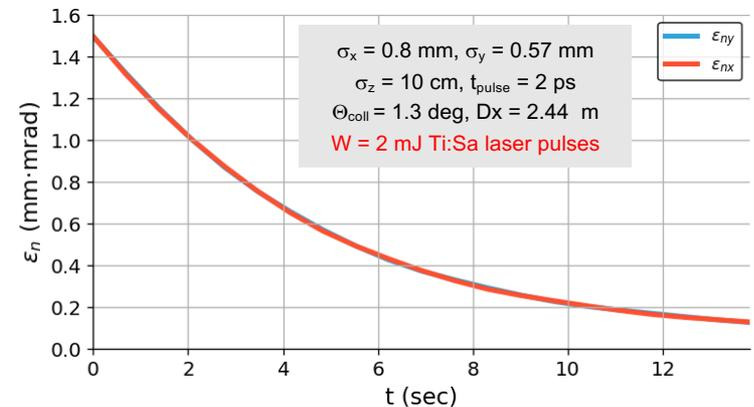
Simulation of laser cooling of the lithium-like  $\text{Ca}^{17+}$  bunches in the SPS: **transverse emittance evolution**.
