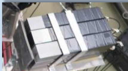
PARIS and LaBr3 high-energy \gamma -ray array
