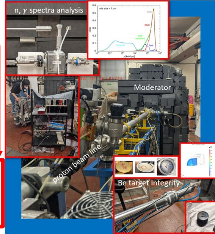
**Test of neutron converter for accelerators, materials**
