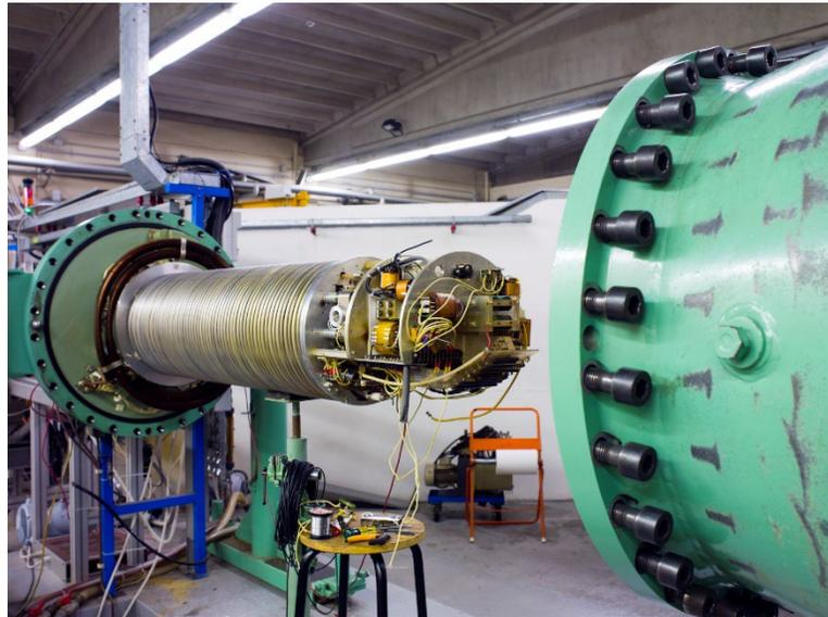
Van der Graaf accelerator type. Light ions with 2 MV terminal voltage
