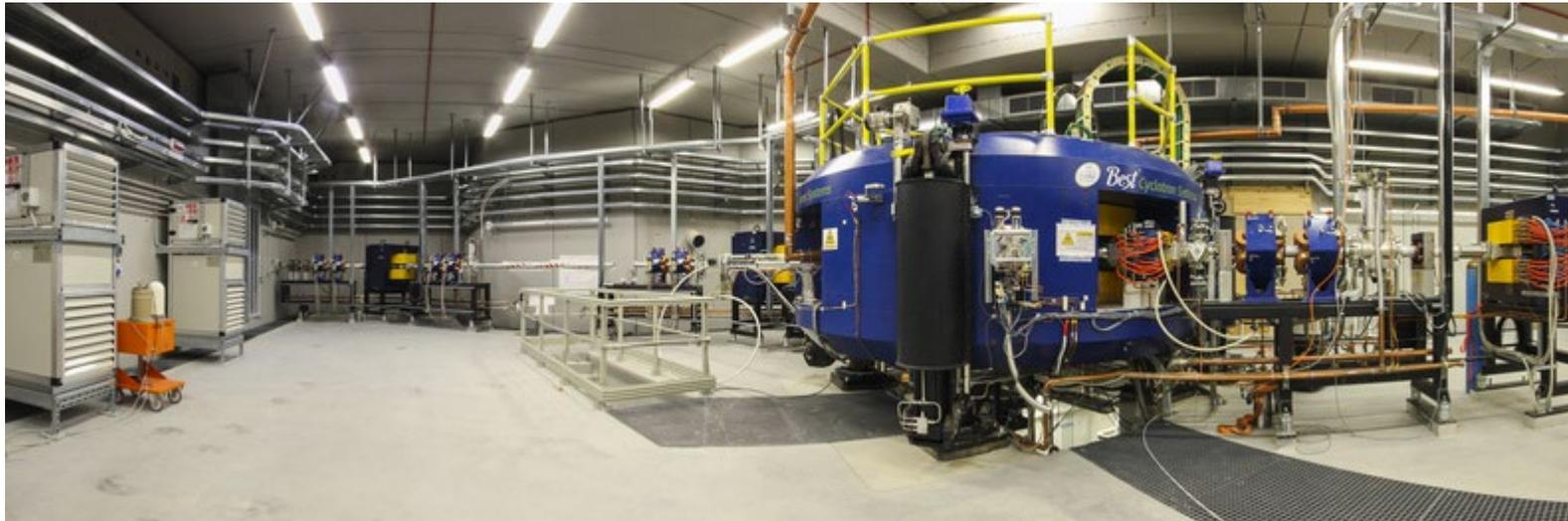
Normal conductive cyclotron with double extraction lines (70 MeV protons at 800  $\mu$ A). It is under commissioning, and it will be equipped with eight target stations. Main stations here
