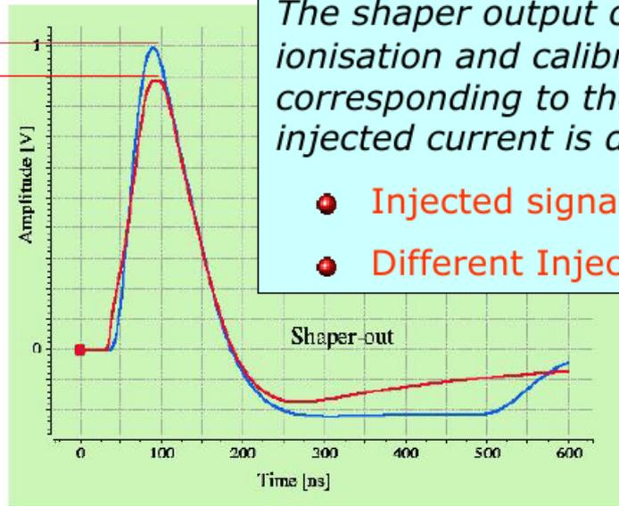
The shaper output of the ionisation and calibration signal corresponding to the same injected current is different!
