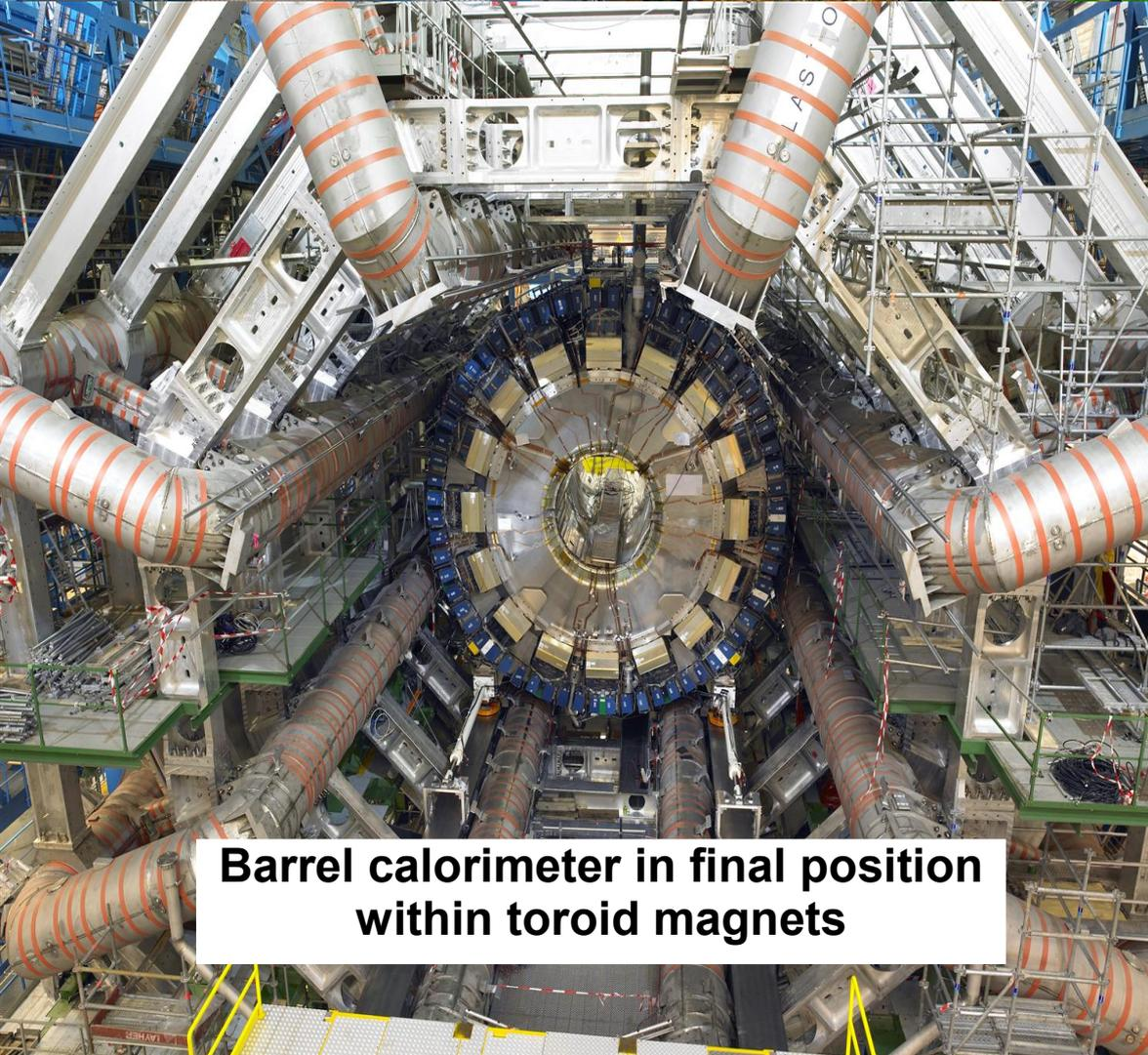
Barrel calorimeter in final position within toroid magnets
