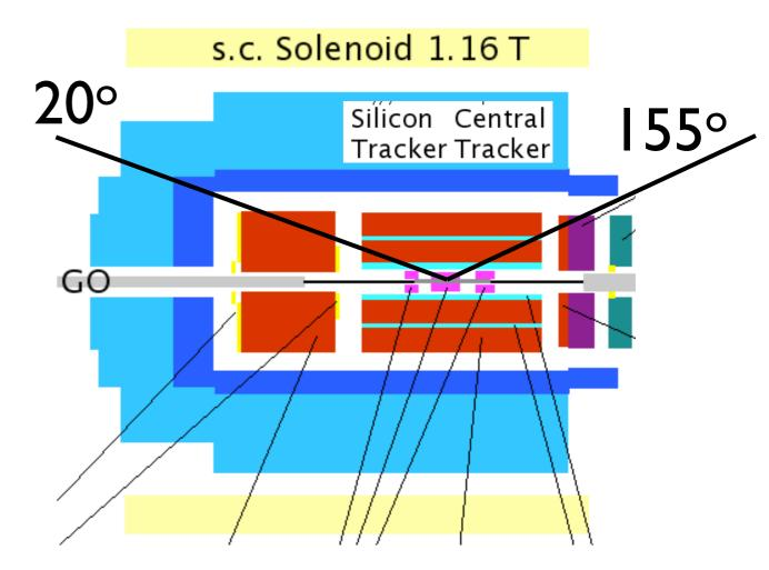
quark scattering angle,  $\theta_{q,lab}$ , calculated from kinematics. Ensures current region of Breit frame remains within tracking acceptance. Easy to calculate in theory!
