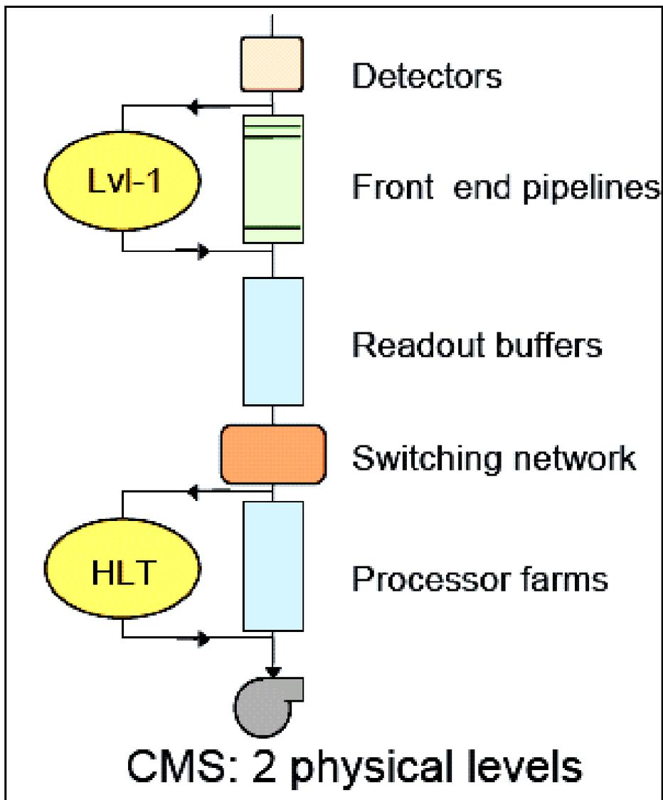
CMS Trigger system consists of two levels:
