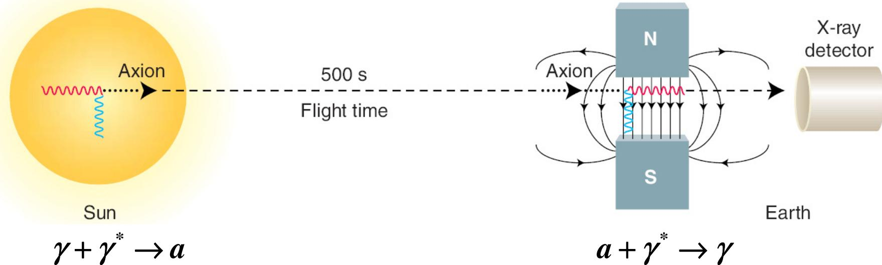
$$P_{a \rightarrow \gamma} = \left( \frac{B g_{a\gamma}}{2} \right)^2 \frac{1}{q^2 + \Gamma^2/4} [1 + e^{-\Gamma L} - 2e^{-\Gamma L/2} \cos(qL)]$$
