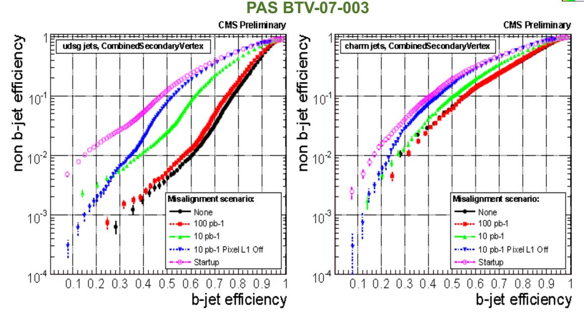
CMS has already been aligned with cosmic data with a precision corresponding to the 10 pb<sup>-1</sup> scenario!
