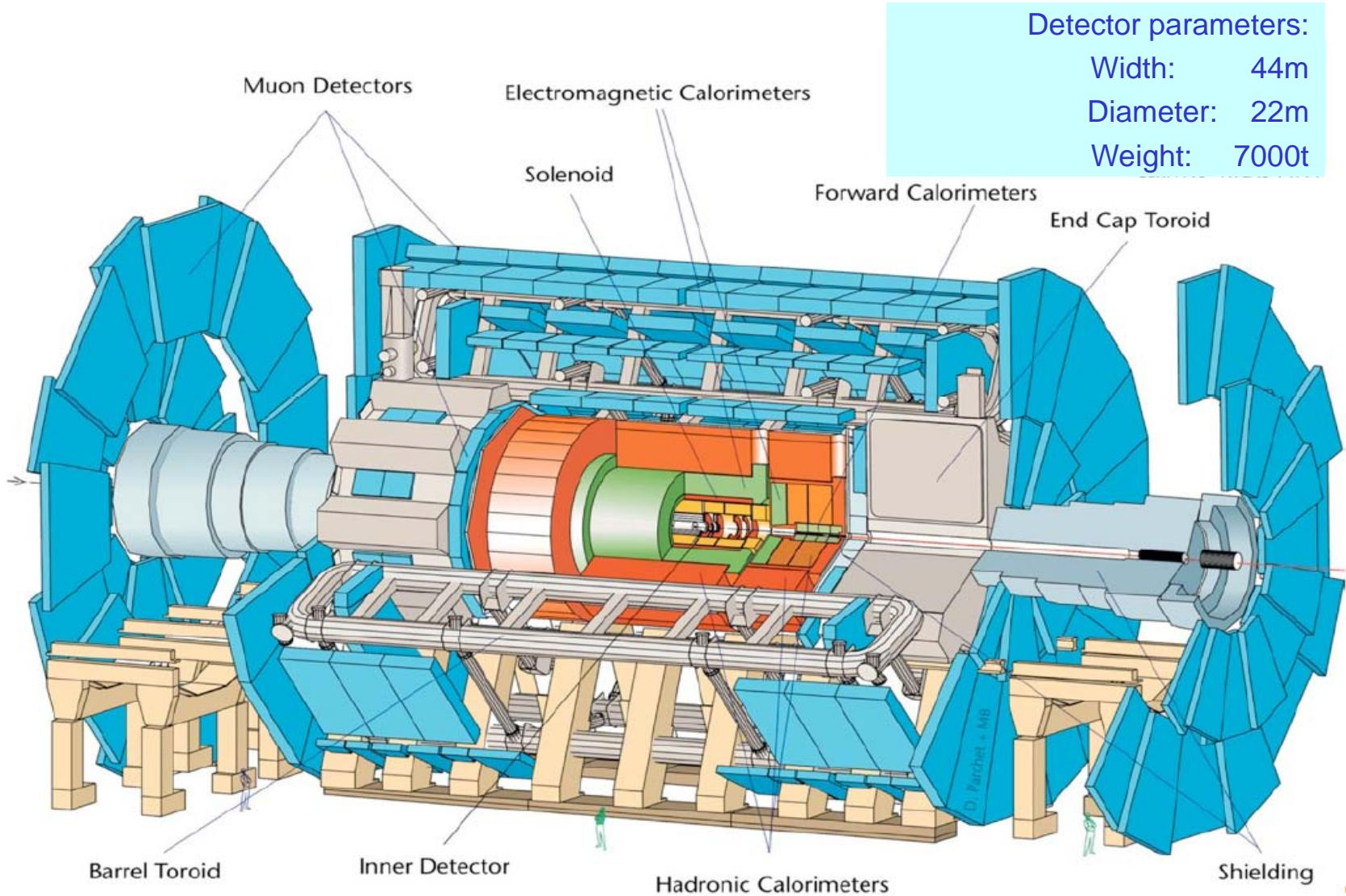
Inner tracker, EM and hadronic calorimeters, muon spectrometer
