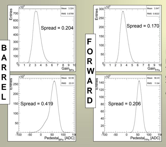
For each pixel, gain and pedestals are determined from a linear fit to the gain response function. There are dedicated gain calibration runs.
