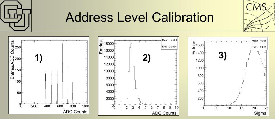
For each hit (above threshold), the pixel address is encoded with six analogue levels over five clock cycles (the sixth cycle gives the pixel charge). The histograms above show:
