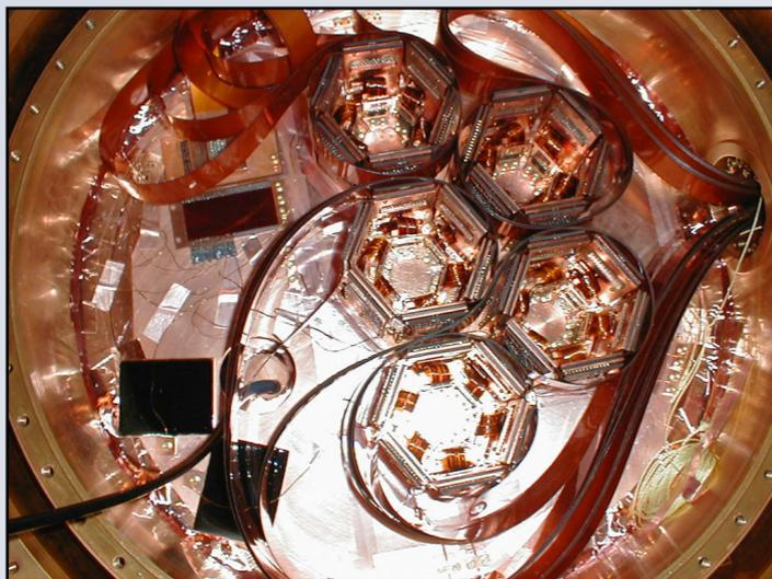
**Control Backgrounds** by going underground, using clean materials and shielding
